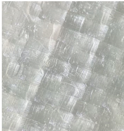
Figure 5: The bubbly texture and misaligned fibers in the sheet layup
