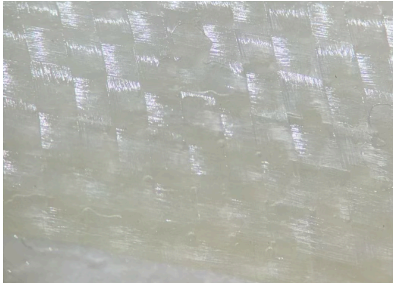
Figure 7: Air bubbles in the tube layup
