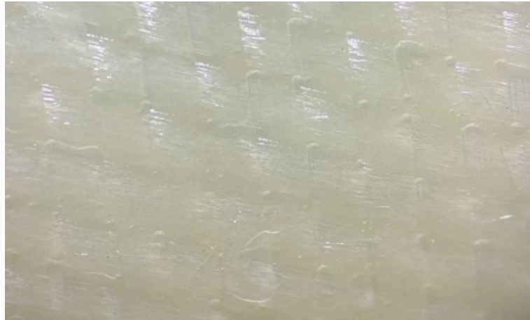
Figure 8: Air bubbles and discoloration in the tube layup
