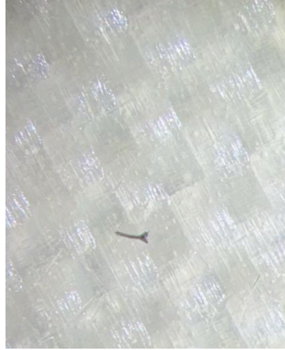
Figure 4: A dark-colored speck and misaligned fiber in the sheet layup
